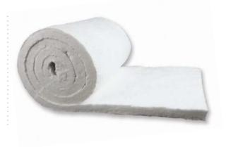
NUTEC Fibratec\* ceramic fiber blanket is composed of long, flexible, interwoven fibers manufactured by the "blown" and the "spun" process yielding a strong, lightweight yet durable blanket for applications in a temperature range from 538°C (1000°F) to 1480°C (2700°F).
