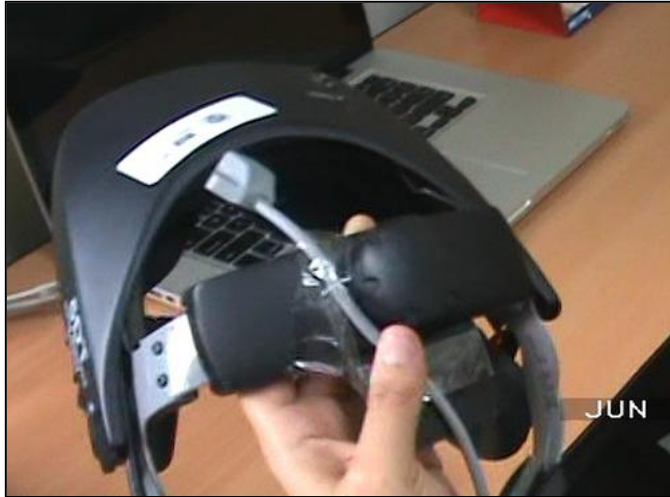
Figura 5.9 Sensor adjunto al head mounted display 5DT
