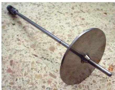
**Figura 3.33 Spindle RV-2.**
