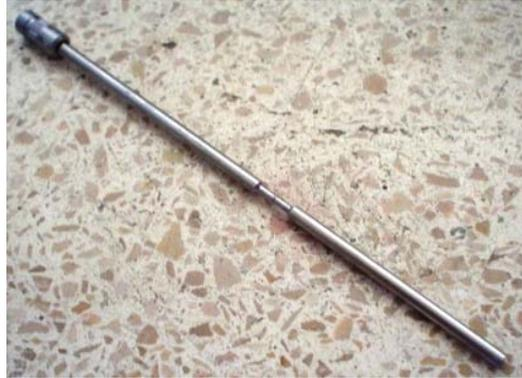
**Figura 3.18 Spindle RV-7.**
