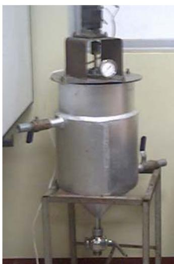
Figura 3.1 Bioreactor
