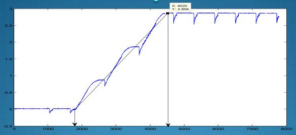
Voltaje inicial = 0 Voltaje final = 2.85 Valor del paso = 2.85 63% = 1.79V (x) = 1.79 X = 3.29 Seg.
