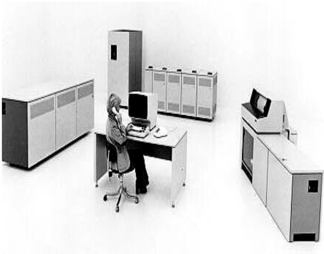
*Figura 1.1 Mainframe IBM-4341*
