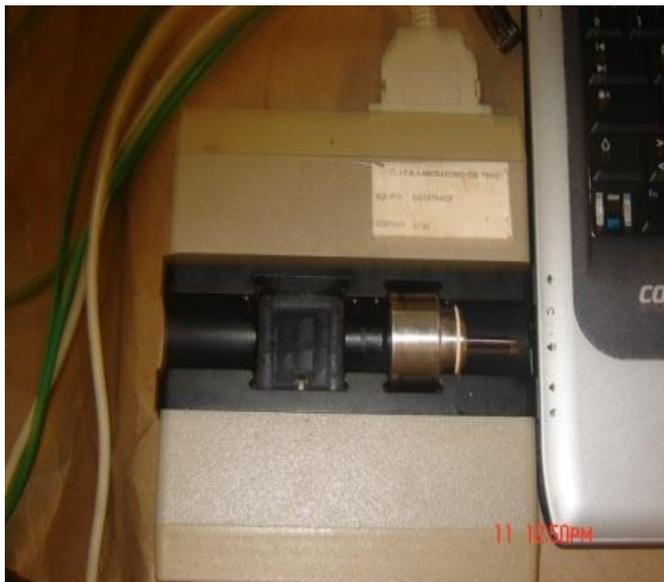
**FIGURA 2.6 PC INTERFACE SYSTEM DATATRACE<sup>®</sup>**
