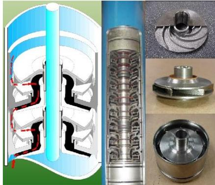
Figura 2.10 Bomba electro sumergible
