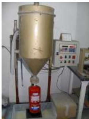
**FIGURA 7.9 RECARGA DE EXTINTOR CON POLVO.**
