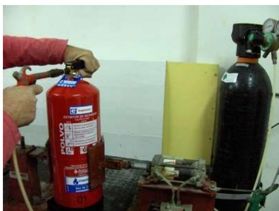
**FIGURA 7.11 RECARGA MANUAL DE NITRÓGENO.**
