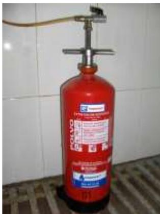
**FIGURA 7.6 FASE EN LA QUE EL EXTINTOR SE LLENA CON AGUA.**
