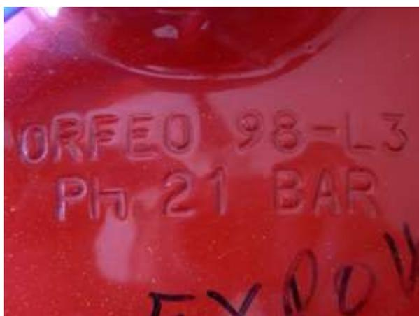
**FIGURA 7.3 MARCADO PH SOBRE EXTINTOR**
