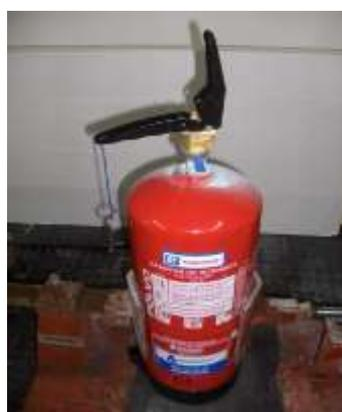
**FIGURA 7.4 EXTINTOR CON LA VÁLVULA DESENROSCADA.**
