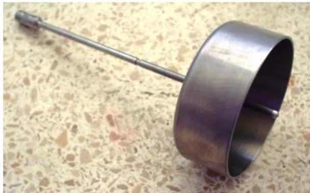
**Figura 3.31 Spindle RV-1.**
