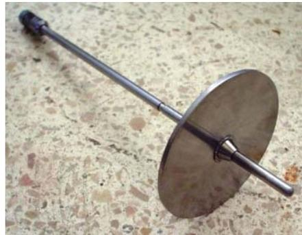
**Figura 3.33 Spindle RV-2.**
