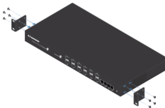
Attaching Rack-Mount Brackets to the EdgeSwitch XG
