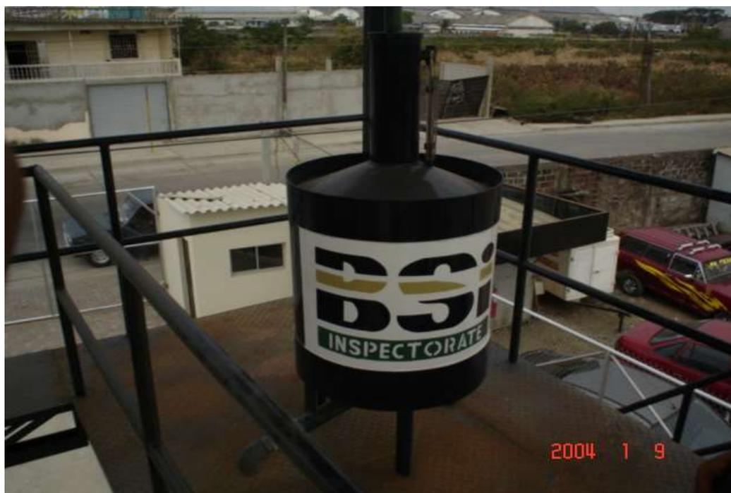
**FIGURA 1.3 PATRON VOLUMETRICO DE 50 GL.**
