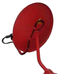
Figura 4.16 Lazo de cable coaxial [36]
