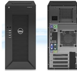
Figura 2.37. Servidor Dell PowerEdge T30 – Intel Xeon.
