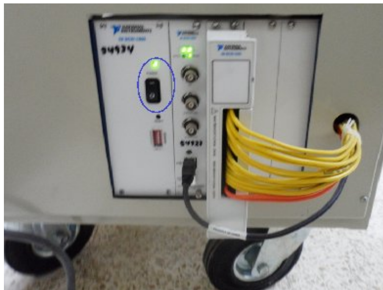
Figura A - 18 Chassis NI-SCXI 1000
