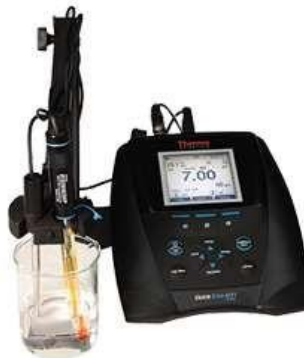
Figura G.6 PH-meter Thermo Scientific Orion Star™ A211 Fuente: Thermo Scientific Orion Star™ and Star Plus Meter User Guide
