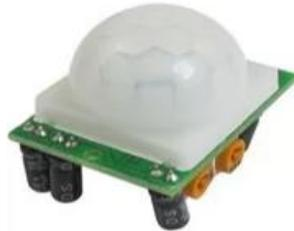
Figura 3.5 Sensor de Movimiento PIR HC-SR501 [8]
