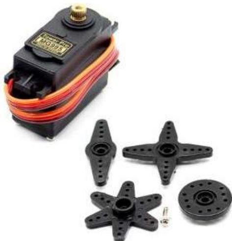
**Imagen 2.10 Servomotor MG995 (Nextia FENIX , Servomotor)**
