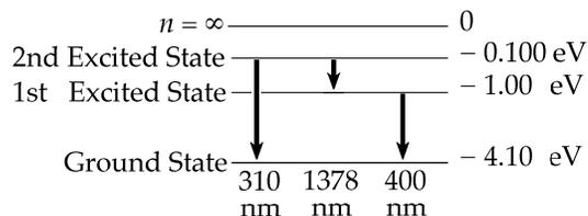
The energy level diagram having the fewest levels and consistent with these energies is shown at the right.
