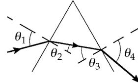
**35.27** Taking  $\Phi$  to be the apex angle and  $\delta_{\min}$  to be the angle of minimum deviation, from Equation 35.9, the index of refraction of the prism material is
