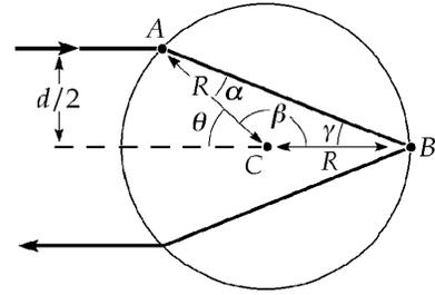
If the emerging ray is to be parallel to the incident ray, the path must be symmetric about the center line  $CB$  of the cylinder. In the isosceles triangle  $ABC$ ,  $\gamma = \alpha$  and  $\beta = 180^\circ - \theta$ . Therefore,  $\alpha + \beta + \gamma = 180^\circ$  becomes
