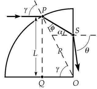
From triangle OPS,  $\phi + (\alpha + 90.0^\circ) + (90.0^\circ - \gamma) = 180^\circ$  or the angle of incidence at point S is  $\alpha = \gamma - \phi$ . Then, applying Snell's law at point S gives  $(1.00) \sin \theta = n \sin \alpha = n \sin(\gamma - \phi)$ , or
