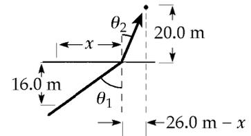
The lifeguard on land travels eastward a distance  $x = (16.0 \text{ m})\tan \theta_1$ . Then in the water, he travels  $26.0 \text{ m} - x = (20.0 \text{ m})\tan \theta_2$  further east. Thus,  $26.0 \text{ m} = (16.0 \text{ m})\tan \theta_1 + (20.0 \text{ m})\tan \theta_2$
