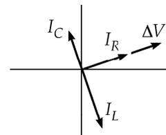
$$33.67 \quad (a) \quad I_{\text{rms}} = \Delta V_{\text{rms}} \sqrt{\frac{1}{R^2} + \left(\omega C - \frac{1}{\omega L}\right)^2}$$
