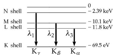
The ionization energy for K shell = 69.5 keV, so, the ionization energies for the other shells are:  $\boxed{\text{L shell} = 11.8 \text{ keV}}$  :  $\boxed{\text{M shell} = 10.1 \text{ keV}}$  :  $\boxed{\text{N shell} = 2.39 \text{ keV}}$
