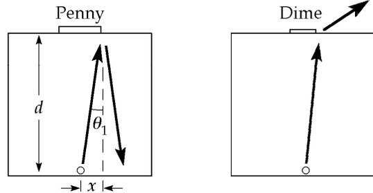
**\*35.42** (a)  $\frac{\sin \theta_2}{\sin \theta_1} = \frac{v_2}{v_1}$  and  $\theta_2 = 90.0^\circ$  at the critical angle
