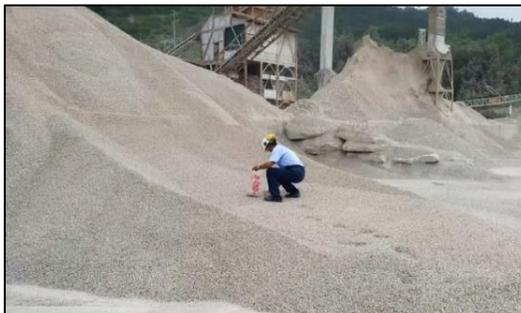
**FIGURA 3.3 TOMA DE MUESTRA EN ACOPIO**
