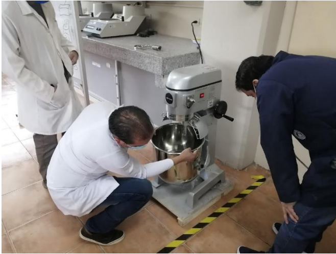
Fig. 3. Preparation of Specimens with the use of a mixer
