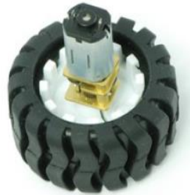
Pololu wheel 42×19mm with micro metal gearmotor.
