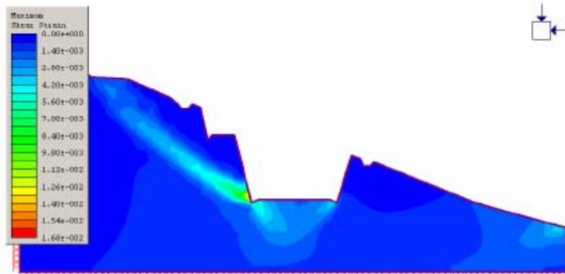
**Figure 4.5 Maximum Shear Strain Contours
