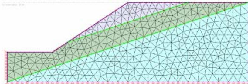
**Figure 1.4 Phase<sup>2</sup> Finite Element Mesh (6-Noded triangles)**
