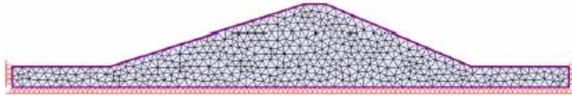
Figure 5.3 Phase<sup>2</sup> Finite Element Mesh (6-Noded triangles)
