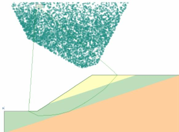
Figure 1.3 Non-Circular Path Search Method, Spencer Method
