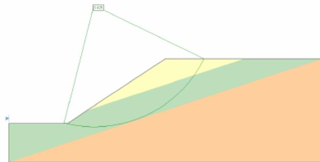
Figure 1.2 Circular Auto Refine Search Method, Spencer Method
