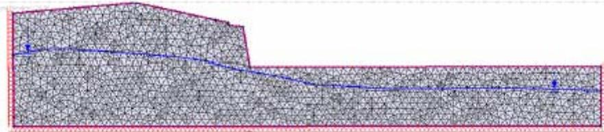
Figure 3.3 Phase<sup>2</sup> Finite Element Mesh (6-Noded triangles)
