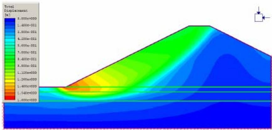
Figure 2.5 Total Displacements Contours (SRF = 1.4)
