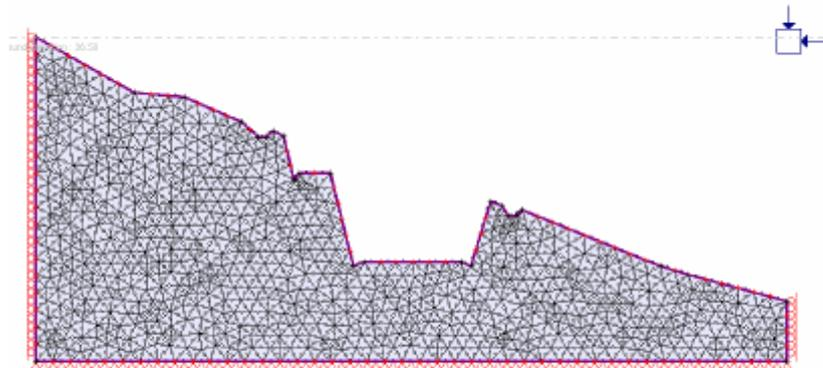
**Figure 4.3 Phase<sup>2</sup> Finite Element Mesh (6-Noded triangles)**
