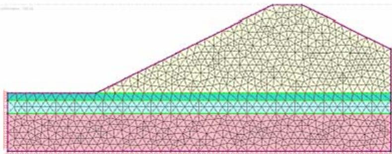
Figure 2.4 Phase<sup>2</sup> Finite Element Mesh (6-Noded triangles)
