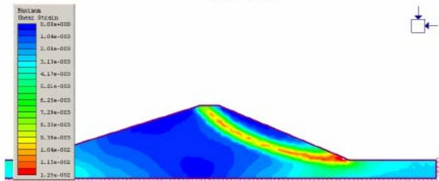
Figure 5.5 Maximum Shear Strain Contours
