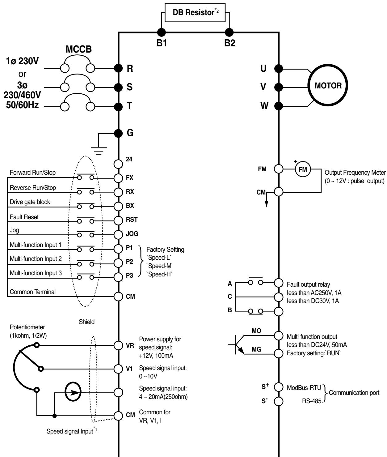
Note) "●" display main circuit terminals, "○" display control circuit terminals.
