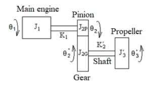
In the following table it has been calculated the forced response, considering the reduction gear, for a frequency 20 rad/sec. If the amplitude of the exciting torque is 24500 N-m, calculate the amplitude of the contact force between the teeth of pinion and gear. (30)
