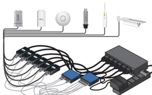
Deployment without TOUGHSwitch
