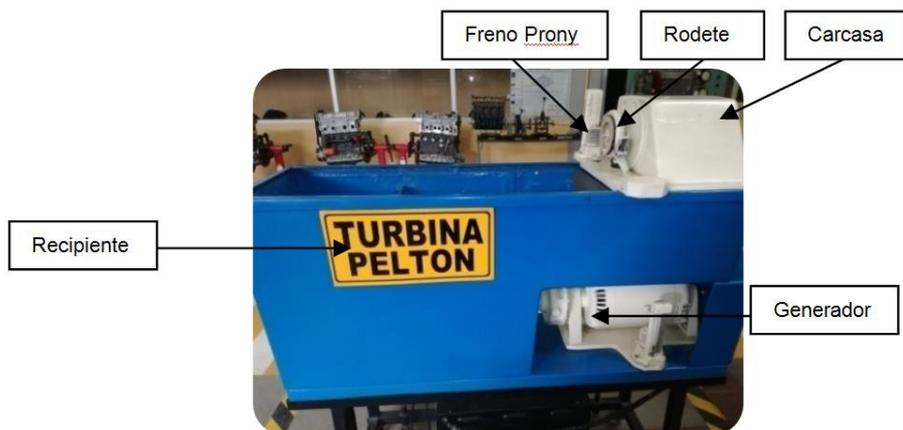
**Figura 1. 6 Turbina Pelton**
