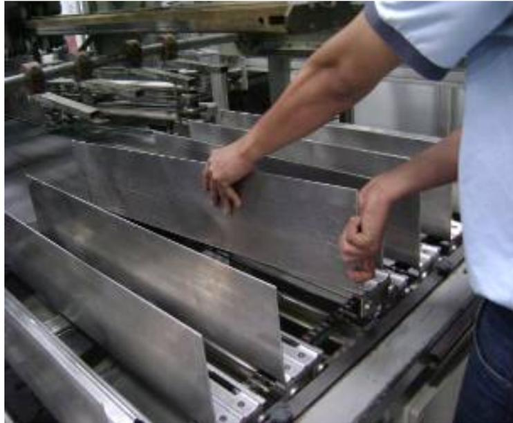
FIGURA 3.5 PALAS DE LA MÁQUINA QWRAP
