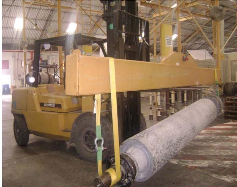
FIGURA 4.5 MONTACARGAS TRANSPORTANDO RODILLO
