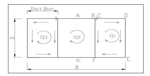
In a preliminary analysis, after performing two cuts in the section, values for the correcting shear flows are  $q'_1$ : -81.3,  $q'_2$ : 0.0 and  $q'_3$ : +81.3 m<sup>2</sup>-mm ( $q'_i$ = $Ic\ q_i/V$ , where Ic is the sectional inertia,  $q_i$  is the correction shear flow and V is the shear force on the section).
