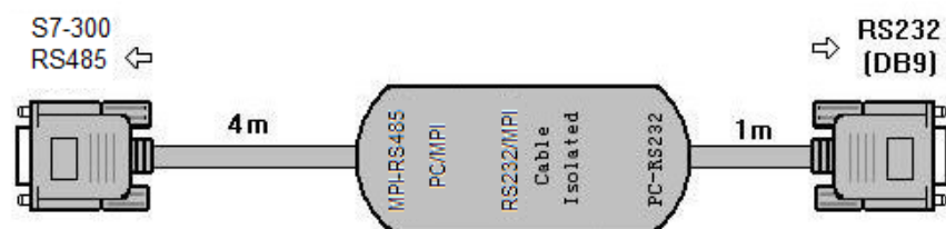
Fig. 3.15. Cable PC - MPI - S7-300. [21]
