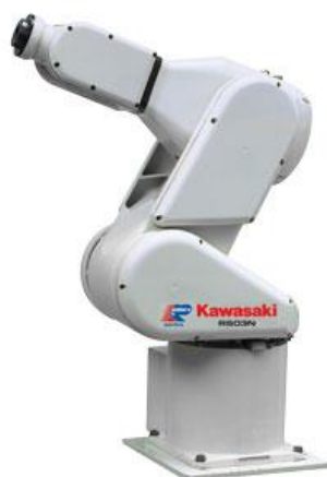
Figura 2.17: Robot industrial Kawasaki RS03N
