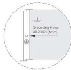
Figure 8: Grounding hole detail
