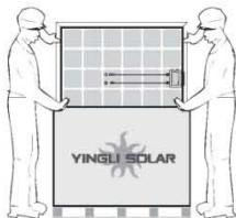
Figure 3: Removing PV modules from a pallet
