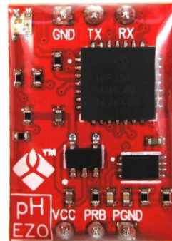
Figura 3.4: EZO™ pH Circuit de Atlas Scientific [12]
