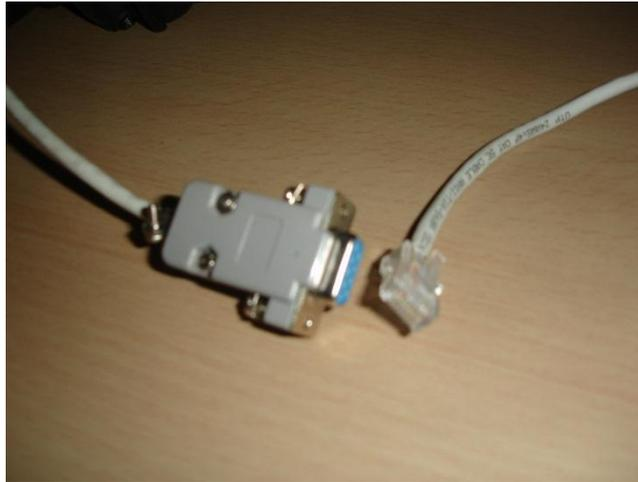
**Figura 2.9: Cable RJ45-MDT 1500**
