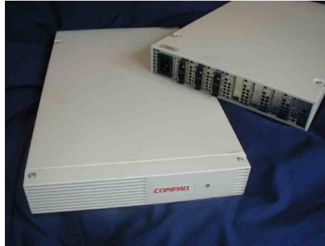
Figura 6.12: Hub de Fibre Channel
