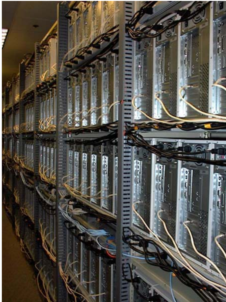
Figura 3.1.3-1. 1000-Pentium Beowulf-Style Cluster Computer [F13]
