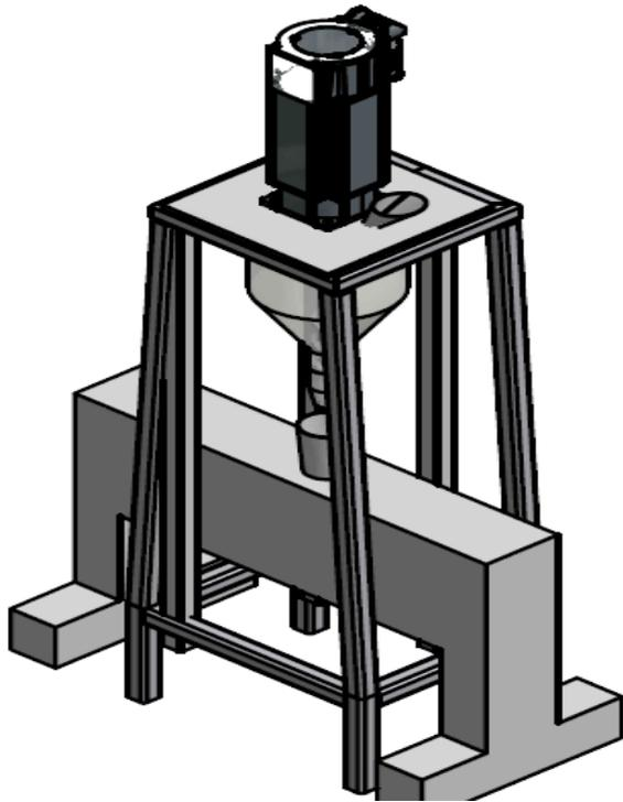
**Figure 6.** Auger filling system design.
