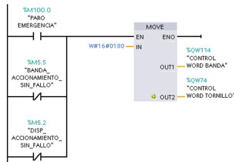
**Figure 15.** Emergency and failure stop's block[1].
