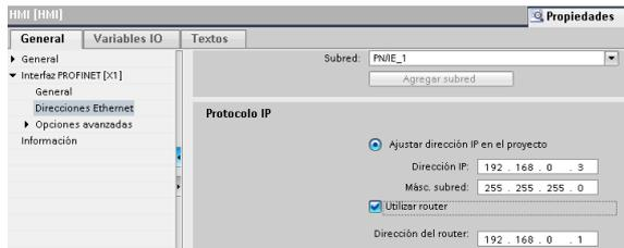
Figure 9. PROFINET configuration for HMI[1].
