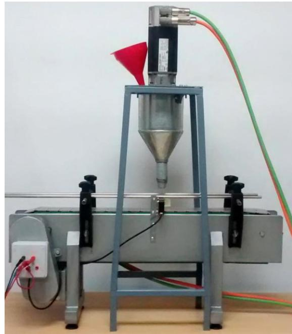
**Figure 7.** Belt conveyor, hopper, photoelectric sensor and servomotor of the auger filling system.
