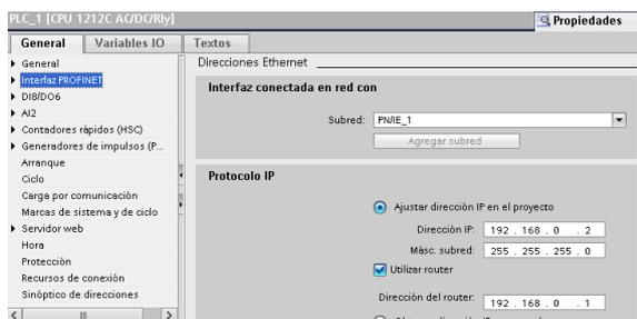
Figure 10. PROFINET configuration PLC[1].
