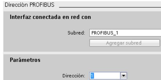
Figure 12. PROFIBUS configuration of the network's master[1].
