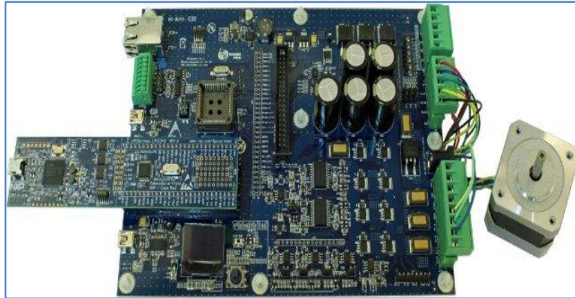
Figura 2.23: Vista LPCXpresso Motor Control Board [15]
