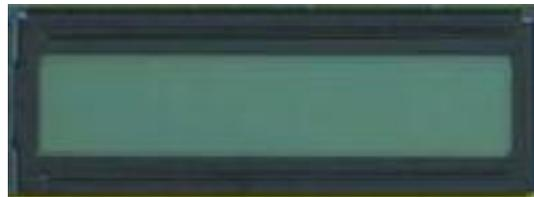
**Figura 2.2 - MÓDULO LCD 16X2 [2]**
