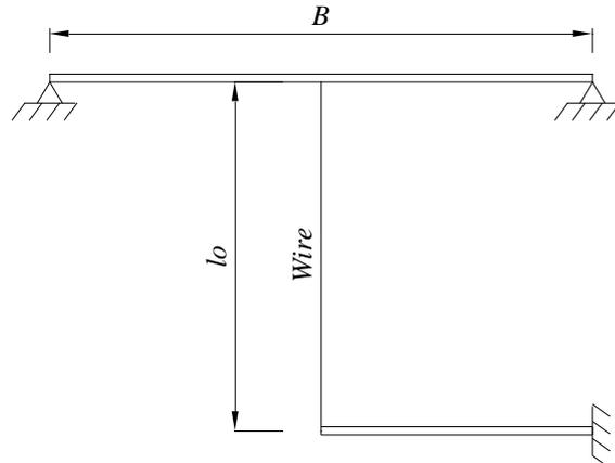
1.04E-5 1/°C. Dimension  $B$ : 1.52 m, and both beams have the following characteristics:  $E$ : 1.06E9 kg/m<sup>2</sup> and  $I_c$ : 5.00E-6 m<sup>4</sup>. Express your answer in kilograms.
