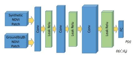
Figure 5.3 – GAN architecture of the second supervised approach for NDVI vegetation index estimation. A single level layer model (flat) evaluated as generator network; bottom the discriminator network.
