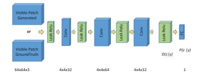
Figure 4.4 – Illustration of conditional GAN (CDCGAN) network architecture, the third proposed approach for NIR image colorization.
