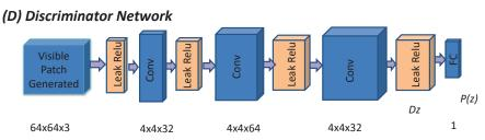
Figure 4.3 – Illustration of the triplet GAN (DCGAN) network architecture, the second approach for NIR image colorization.
