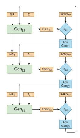
Figure 4.7 - Illustration of the proposed stacked GAN schema used NIR image colorization.
