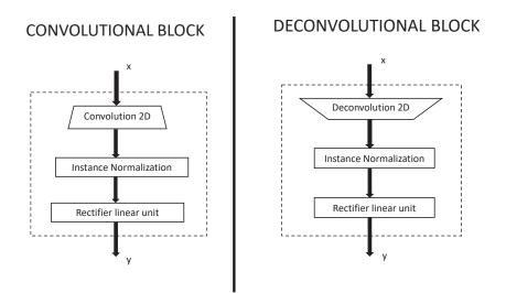
Figure 5.7 – Convolutional and deconvolutional blocks modified to included instance normalization from [39].
