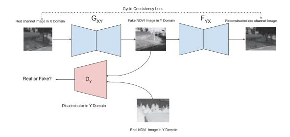
Figure 5.9 – Cycle generative adversarial model *G*:  $X(red channel) \rightarrow Y(NDVI)$  and its discriminator  $D_{\gamma}$ .
