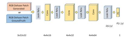
Figure 6.1 – Illustration of the first proposed approach based on triplet dense CGAN architecture used for image dehazing.
