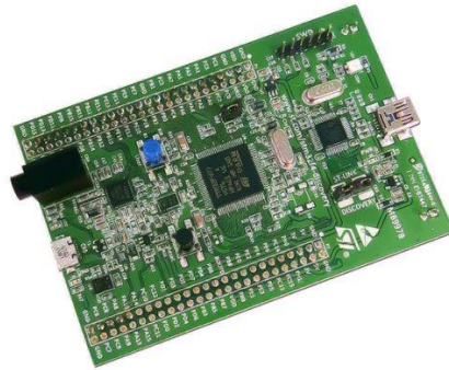
Figura 1.2 Discovery Board STM32F407Vgtx [5]
