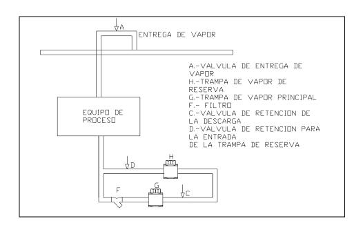
FIGURA 8.8: DIAGRAMA DE TRAMPAS DE VAPOR.
