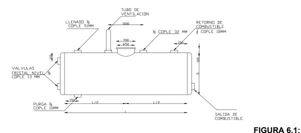
TANQUE DE COMBUSTIBLE PARA DIESEL OIL.
