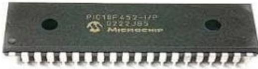
FIGURA 3-2: Microcontrolador PIC18F452-I/P
