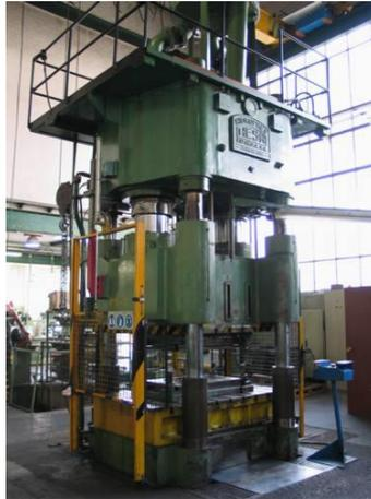
**FIGURA 5.2 PRENSA HIDRAULICA DOBLE EFECTO.**
