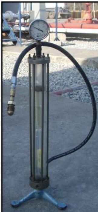
**FIGURA 3.8 HIDRÓMETRO**
