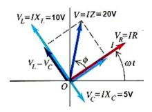
$$\varepsilon^{2} = (V_{R})^{2} + (V_{L} - V_{C})^{2}$$
