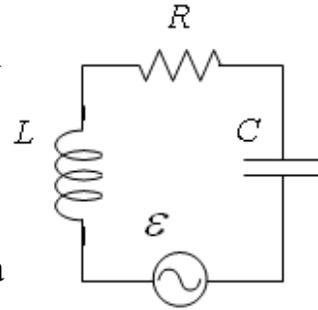
$$\begin{aligned} \varepsilon_{\max} &= 20 \text{ V} \\ I_{\max} &= 2.3 \text{ A} \\ \phi &= +30^\circ \end{aligned}$$
