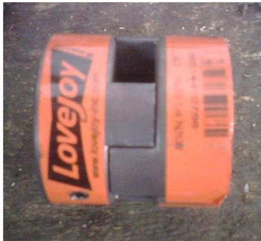
**FIG. 2.4 FOTOGRAFÍA DEL ACOPLÉ SEMIFLEXIBLE**
