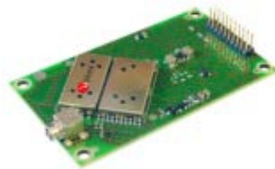
**Figura 9:** Receptor GPS  $\mu$ -Blox RCB-4H
