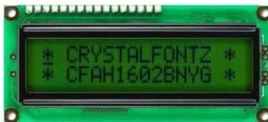
**Figura 13:** Pantalla LCD 16X2
